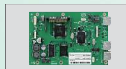
UC-FR5000 (#12) NETWORK CONTROLLER For dPMR Mode 2 multi-site networking
